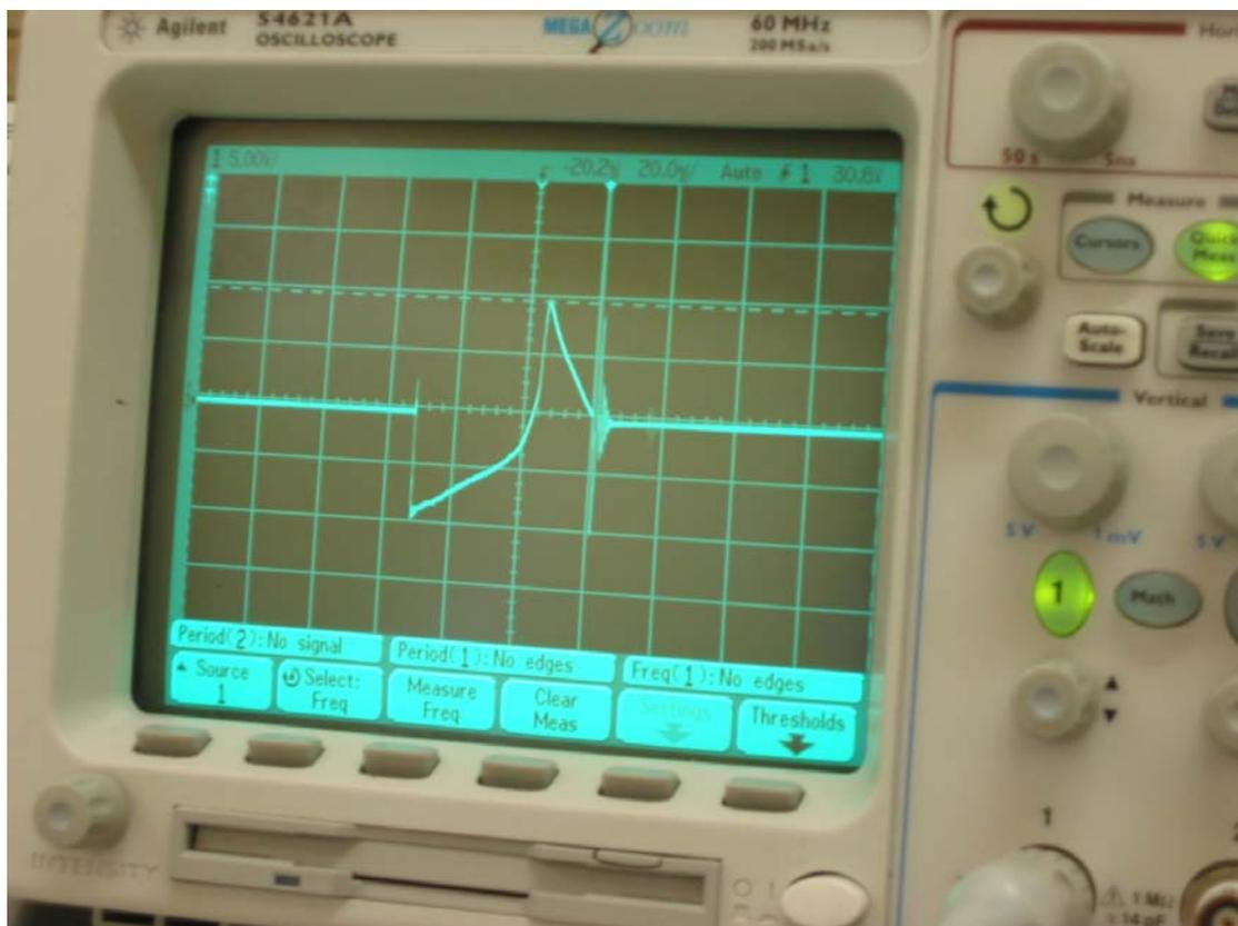
CRO Output of a Single Pulse to the Coil and Collapse.
