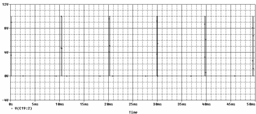
Simulated output from second 555 timer, monostable configuration
