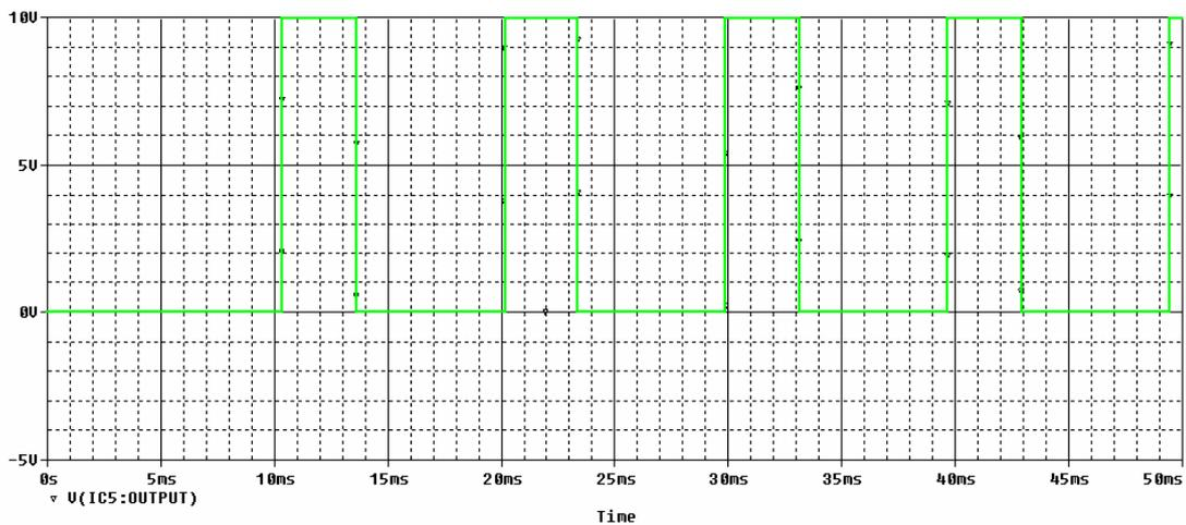
Simulated output of first 555timer; Astable configuration.
