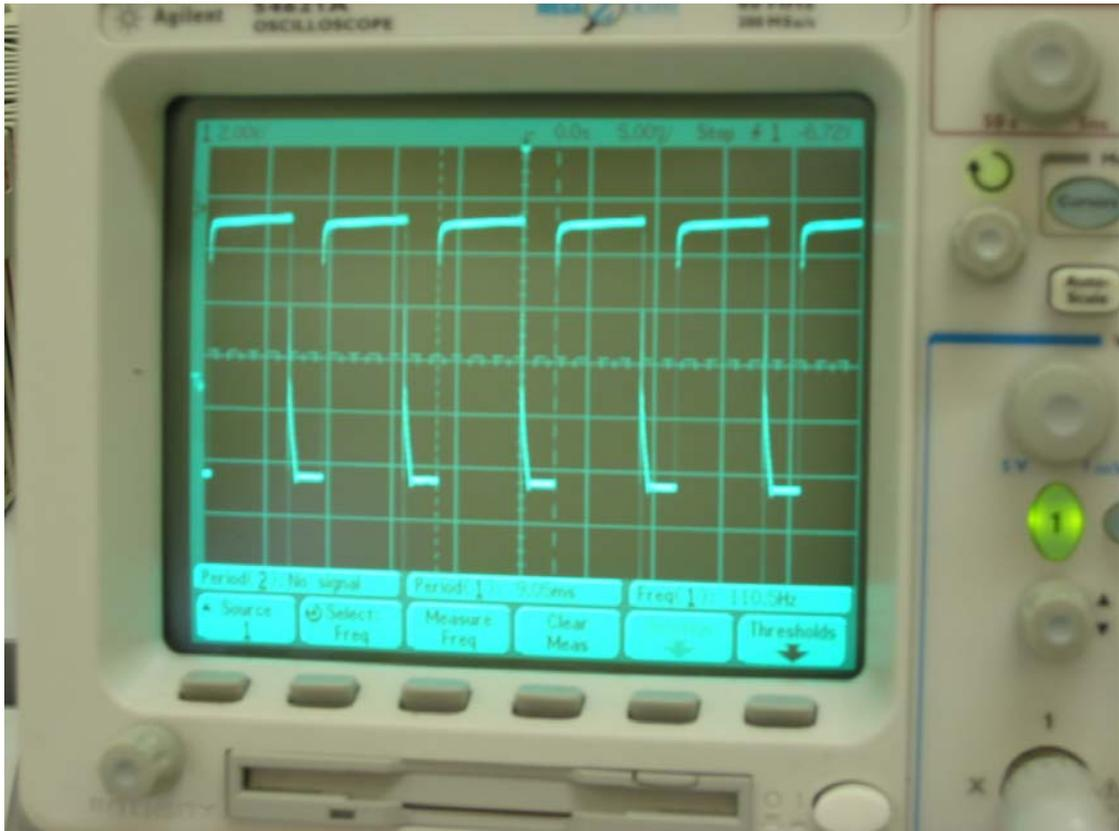
Pulse Train out of IC5, Astable 555 timer output
