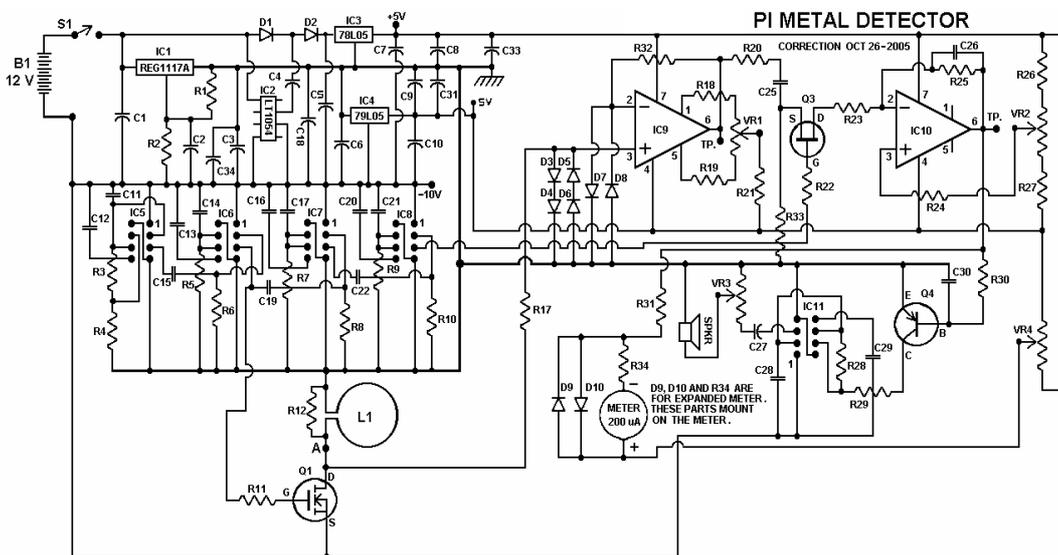
Figure 3 – Schematic of the Pulse 1 Metal Detector
