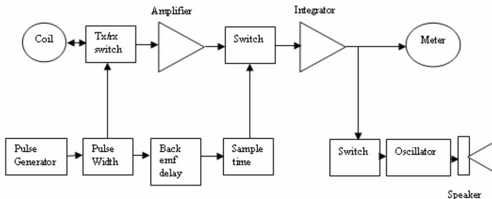
Figure 2 – Block Diagram of the Pulse 1 Metal Detector
