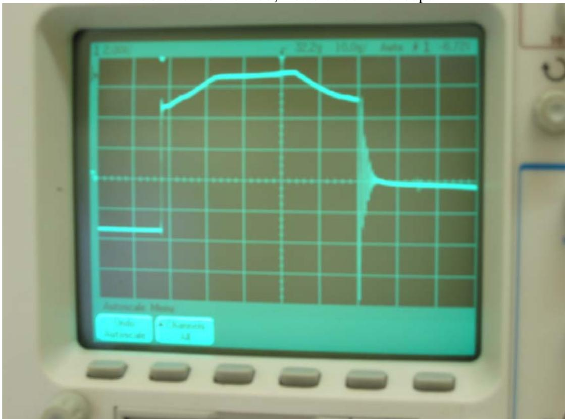
Output from IC6, Second 555 Monostable output.
