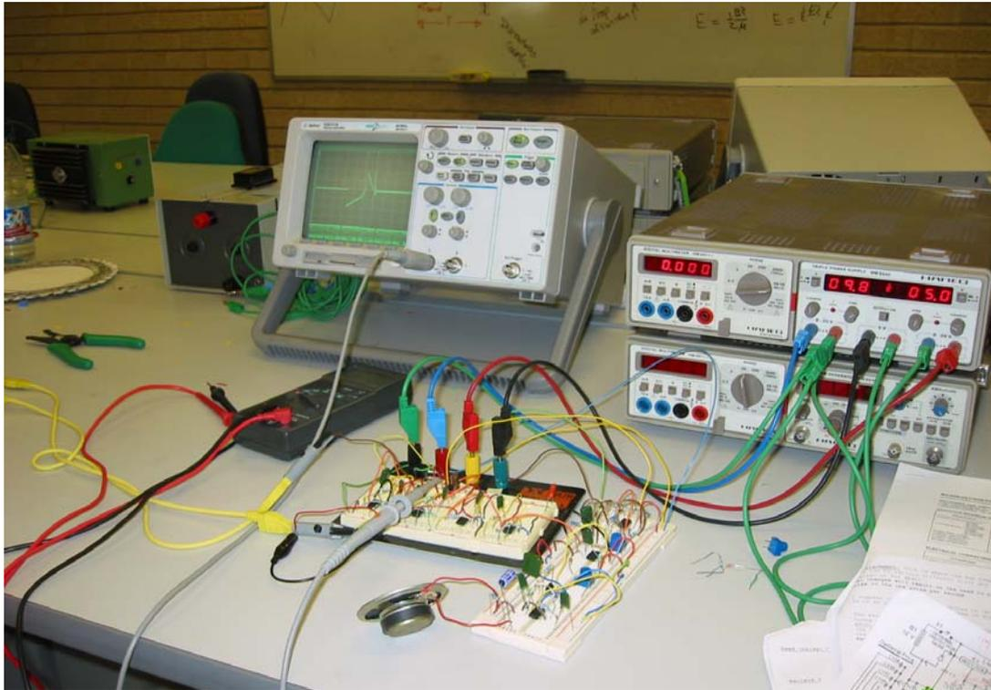
Metal Detector Circuit – Breadboard Implementation.
